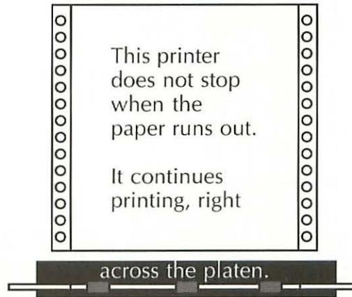
**Probable diagnosis:** The paper error detector is malfunctioning. Most likely, a mailing label got stuck under the platen and the detector arm is jammed by a piece that's still in there.
