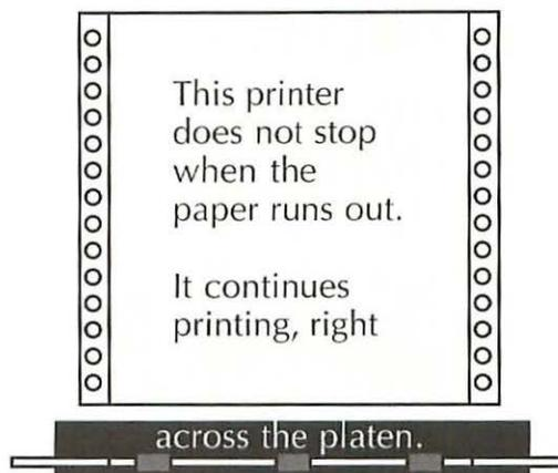
**Probable diagnosis:** The paper empty sensor is malfunctioning. Most likely, a mailing label is stuck under the platen.
