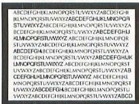
**Probable diagnosis:** The problem is on the H board, located under the control cover plate at the back of the monitor.
